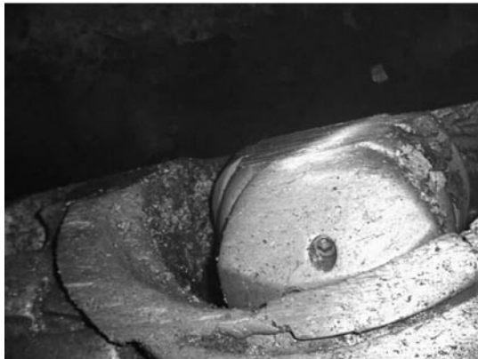
Figure.11 Seriously damaged cutter
