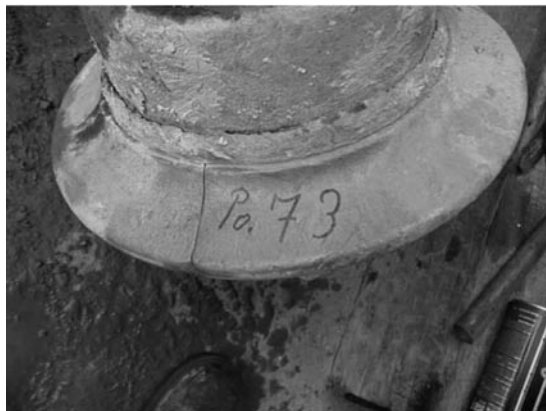
Figure.7 Cutting disk crack by strong impact.
