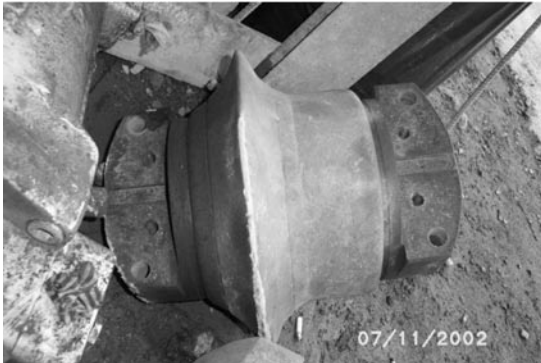
Figure.10 Gauge cutter disk shape from abnormal wear
